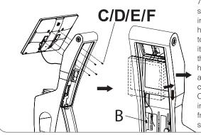
7B. When inserting small cpu, place it into the vertical holder as illustrated to the left by moving it inside the area and then downward into holder. No screws are required but for compatible Lenovo CPUS, you can rotate in two screws (B) from below until securely fastened.
