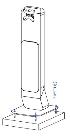
5A. First, find the surface location where you wish to mount the floorstand to. Mark off the locations of the four mounting holes of the base plate.
