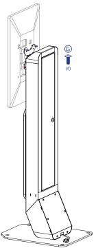
4A. Align VESA holes of display (not included) to the VESA holes of VESA plate of floor stand. Rotate in four screws (G) from behind as shown above using screwdriver tool (not included). Rotate until securely tightened.
