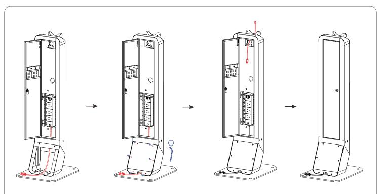
3A. Take the power surge cord (not included) and route it through the base access panel area. Have it come out where there is a notch at the bottom. Take the base access panel cover and place it back on top as shown above. Rotate in the original four integral screws using provided tool (I) until securely tightened.
