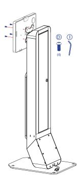
4B. Align VESA holes of enclosure (not included) to the VESA holes of VESA plate of floor stand. Rotate in four screws (D) from the front of the enclosure as shown above using provided tool (I). Rotate until securely tightened. Place device in AFTER you have mounted the enclosure to the foorstand.
