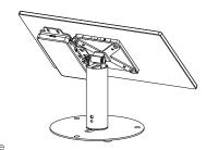
3A. The square bracket (B) has two non-VESA mounting holes available. When mounting in the vertical direction, identify the bracket tab on the long side of the rectangular bracket. Align mounting holes with the square bracket and rotate in the two screws (D) from behind using provided tool (E) until securely tightened.
