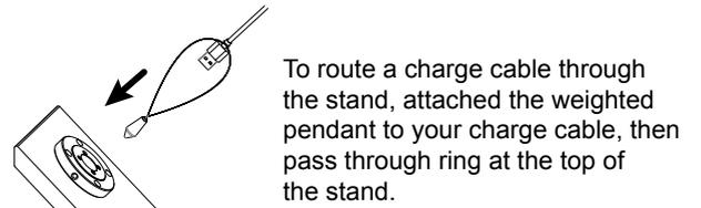
To route a charge cable through the stand, attached the weighted pendant to your charge cable, then pass through ring at the top of the stand.
