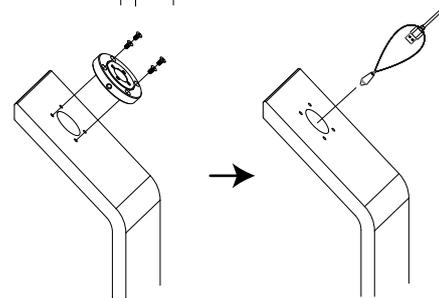
If your cable end is big, remove the ring first and pass the cable with weighted pendant directly through the opening.
