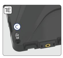
1E. Tighten 4 security screws (C) with the included specialty allen key tool (D). Rotate until securely tightened for all four locations.
