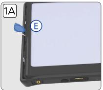
1A. Peel the TPU sleeve from the internal hard case using component (E). Do not take off completely. Peel back enough so you can see the edges of the hard interior case(A)
