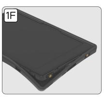
1F. Reinstall the external sillicone rubber sleeve jacket. Start with one corner and work your way around. Using your hands, stretch the sillicone jacket back over the edges to fit properly.
