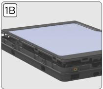
1B. To open case apply gentle pressure to the small clips around the perimeter of the interior hard case. Use your fingers to unclip. The internal hard case will open when all 4 sides are unclipped. Remove the top cover for now.
