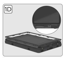
1D. Once the tablet device is inside, plug the internal charging cable into the power socket of the device. Then re-clip back on the front hard cover on top of the hard case. Make sure to go around the perimeter and clp it all in.
