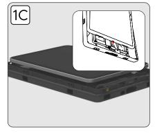
1C. Before inserting your tablet into the case, connect the internal USB-C cable in the case to the charging port on your tablet. After the cable is connected, insert the tablet into the back part of the hardshell case, making sure that the cable connecting your table to the case is neatly routed below the tablet.
