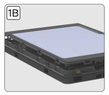
1B. Use the provided pick tool (B) to undo the clips around the perimeter of the hardshell case. If security screws are installed on the rear corners of the case, remove these first with the provided M3 security key (D) before undoing the case clips. Once all of the clips are undone the top part of the hardshell case can be removed.
