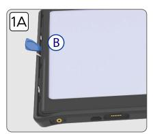
1A. Remove the outer silicone sleeve from the internal hardshell case using the provided pick tool (B)
