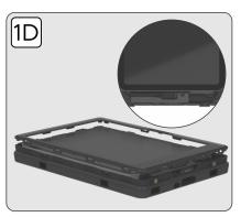
1D. Once the tablet is installed, the top of the hardshell case can be reattached to the bottom of the case. Make sure to check that all case clips around the perimeter are properly secured.
