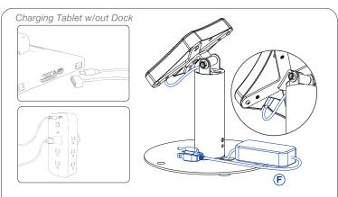
3A. Connect the power supply (F) to an outlet on one end and to the dock as shown above. You want to route the cable through the kiosk/mount body. The tablet case can also be powered directly via USB-C or POGO PIN if needed to charge without the induction dock.
