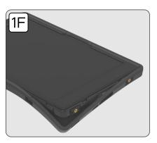
1F. Reinstall the external sillicone rubber sleeve jacket. Start with one corner and work your way around. Using your hands, stretch the sillicone jacket back over the edges to fit properly.
