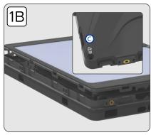
1B. To open case, first make sure the four specialty screws (C) are removed from the back of the hard case using provided tool (D). Then use your fingers or pick (E), to unclip around all edges. The internal hard case will open when all 4 sides are unclipped. Remove the top cover.
