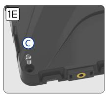
1E. Tighten 4 security screws (C) with the included specialty allen key tool (D). Rotate until securely tightened for all four locations.
