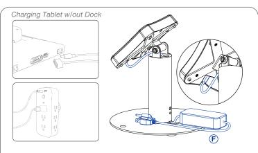
3A. Connect the power supply (F) to an outlet on one end and to the dock as shown above. You want to route the cable through the kiosk/mount body. The tablet case can also be powered directly via USB-C or POGO PIN if needed to charge without the induction dock.
