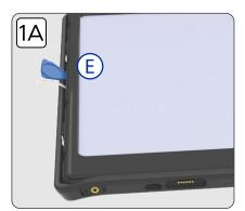
1A. Peel the outer sillicone sleeve from the internal hard case using component (E). Do not take off completely. Peel back enough so you can see the edges of the hard interior case(A).
