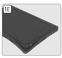
1E. Reinstall the external sillicone rubber sleeve jacket. Start with one corner and work your way around. Using your hands, stretch the sillicone jacket back over the edges to fit properly.
