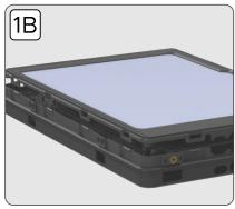
1B. Use your fingers or pick (E), to unclip around all edges. The internal hard case will open when all 4 sides are unclipped. Remove the top cover.
