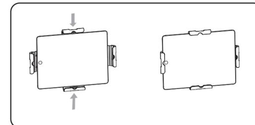
While holder is in 'unlocked' mode, extend the arms outwards until tablet fits comfortable in place. Retract arms until they hold the tablet firmly. Tablet holder can accommodate tablets in cases as well up to 1" thick.
