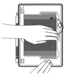
2. While holding the plastic portion of the case with one hand, pull out the folded kickstand carefully with other hand.
