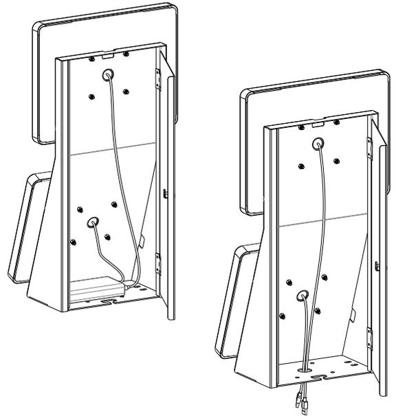
3A. Unlock back storage area using the keys (G). Fish through the holes your cable as shown into the back storage area. Either fish through the holes at the bottom if required or even connect to any small charging items, device or accessories as needed that can fit into the space.
