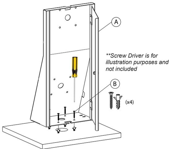
1A. When mounting into a surface for a desk mount mode, use (4) screws and (4) anchors as illustrated (B) and rotate through desk mount (A). Using a screwdriver (not provided), rotate in until securely tightened as shown above.
