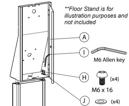
1B. When mounting into CTA Digital's ADD-PARAFS2 stands, first open the back door to the storage area. Then use the provided allen key tool (I) and rotate in screws (H) on top of the washers (J) as shown until securely fastened. Shut door and lock with key. (G)
