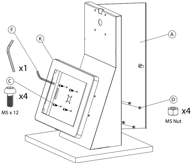
2A. Align VESA holes of CTA's enclosure (K) with one set of the desk mount (A) VESA holes in landscape orientation. Using the included allen key tool (F), rotate in screws (C) while holding hex nut (D) on the back side until securely tightened. Repeat the process for the other set of VESA holes and other enclosure.
