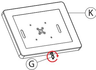
4A. Lock or unlock your tablet enclosure (K) with security key (G) as shown. Make sure to do a full 360 degree rotation before removing.
