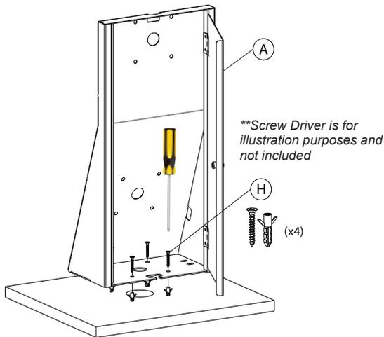
1A. When mounting into a surface for a desk mount mode, use (4) screws and (4) anchors as illustrated (H) and rotate through desk mount (A). Using a screwdriver (not provided), rotate in until securely tightened as shown above.
