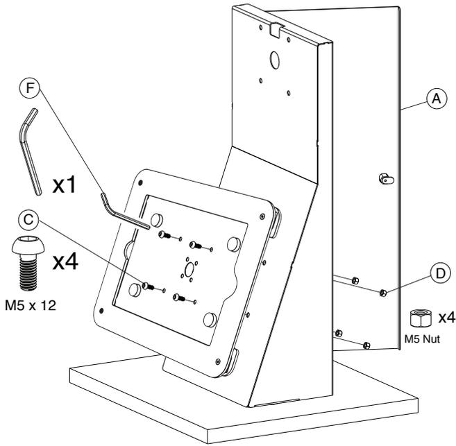
2A. Align VESA holes of CTA's acrylic enclosure (B) with one set of the desk mount (A) VESA holes in landscape orientation. Using the included allen key tool (F), rotate in screws (C) while holding hex nut (D) on the back side until securely tightened. Repeat the process for the other set of VESA holes and other enclosure.
