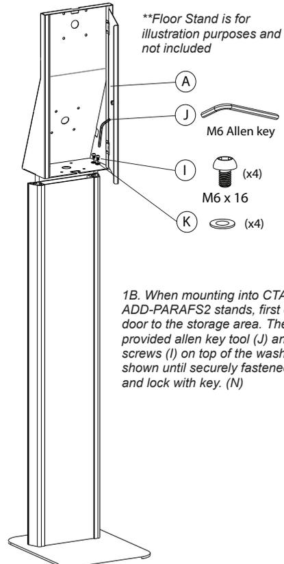
1B. When mounting into CTA Digital's ADD-PARAFS2 stands, first open the back door to the storage area. Then use the provided allen key tool (J) and rotate in screws (I) on top of the washers (K) as shown until securely fastened. Shut door and lock with key. (N)
