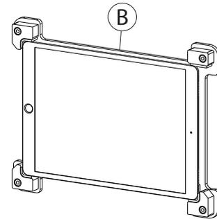
4A. While holding the back security star key (D) tight in place Turn the front security star key (D) counter clock-wise until all 4 screws (B) are unscrewed. Then take off front part of enclosure.
