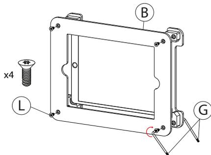
4C. Take the detached enclosure top (B), align the corner holes with the bottom portion. Then use the provided security star key (G), turn in clock-wise the star screws until securely tightened while holding the security star key (G) on the other side with your other hand. Screw in until securely tightened.
