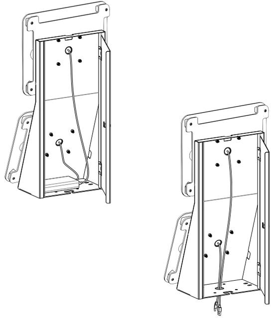
3A. Unlock back storage area using the keys (N). Fish through the holes your cable as shown into the back storage area. Either fish through the holes at the bottom if required or even connect to any small charging items, device or accessories as needed that can fit into the space.
